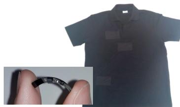
Piezoelectric textile fibers for connected clothes (low power flexible electronics and integrated antennas)
